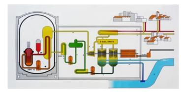
In the two steam generators, the heat generated in the reactor is released into a second circuit. Here, the water is completely sepa-rated from the first circuit and comes to the boil at lower pressure. The resultant steam is channelled on to the turbines which drive the generators.
