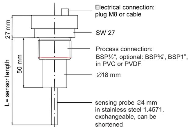
Min. length L from sealing face = 60 mm
